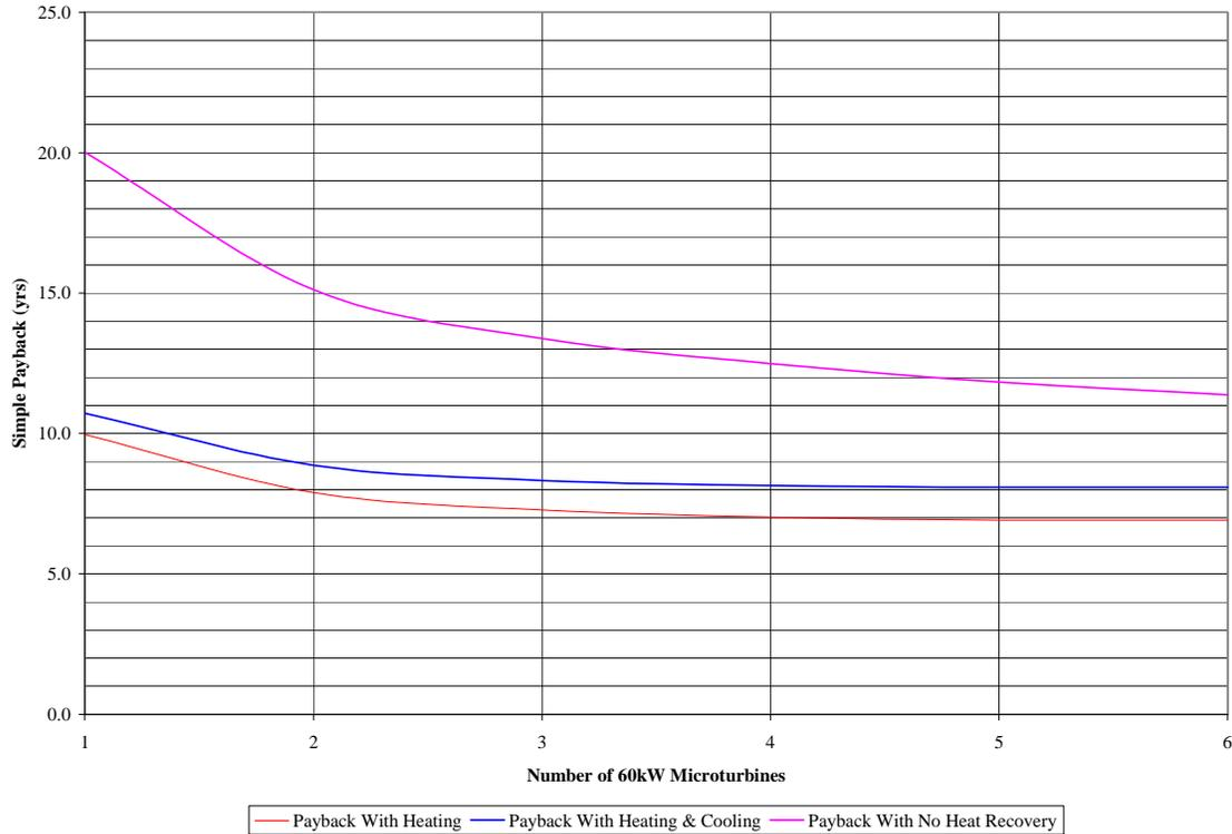
**Figure 7-1 Effect of Number of Microturbines on Simple Payback Period**
