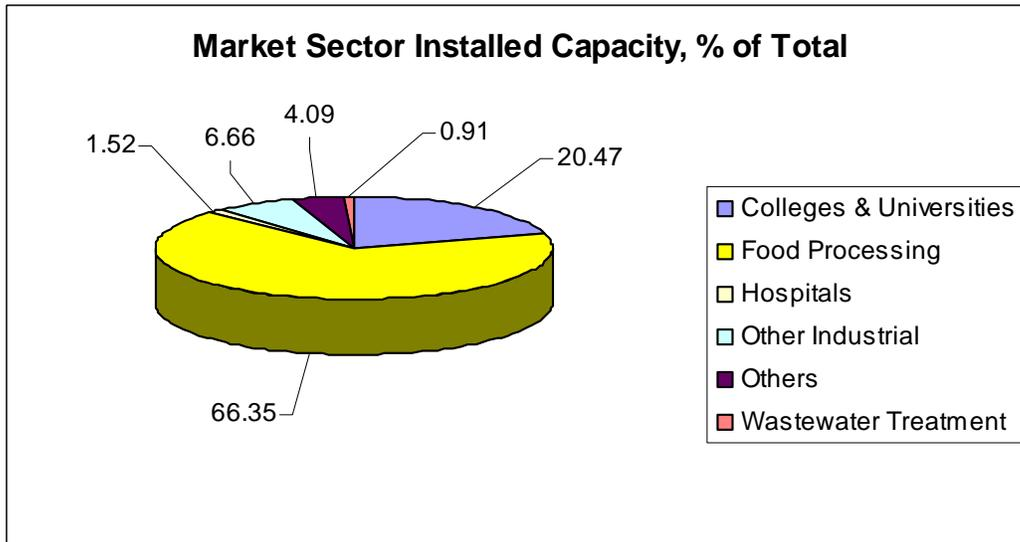
**Figure 3-2 Installed CHP Capacity Share by Market Sector in Iowa**
