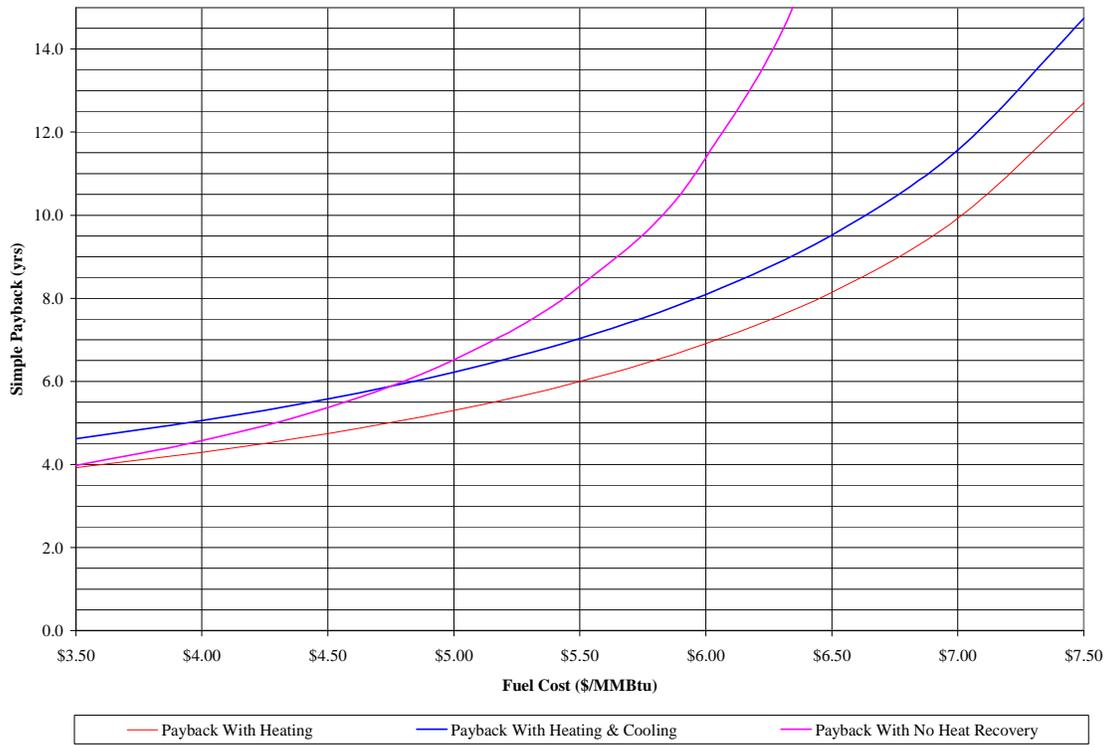
**Figure 7-2. Effect of Fuel Cost on Simple Payback Period**
