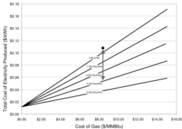
The point is well above the 4,500 Btu/kW line and the system should be left on. **NOTE:**
