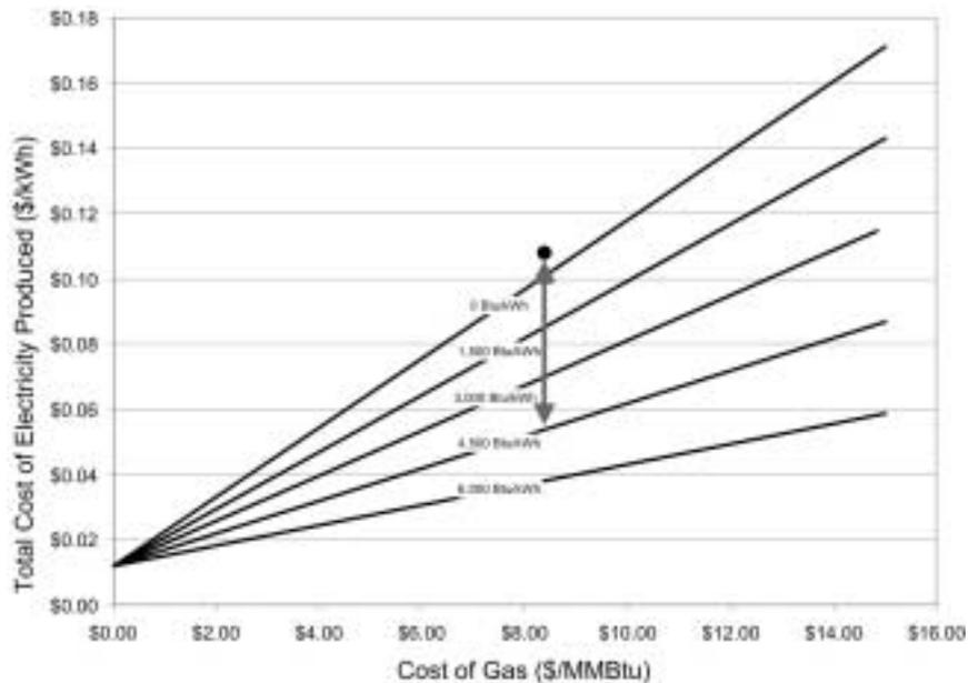
The point is well above the 4,500 Btu/kWh line and the system should be left on.
