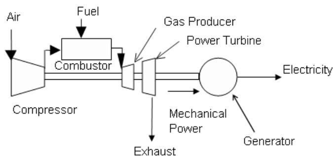
Figure 2. Components in a simple cycle gas turbine.
