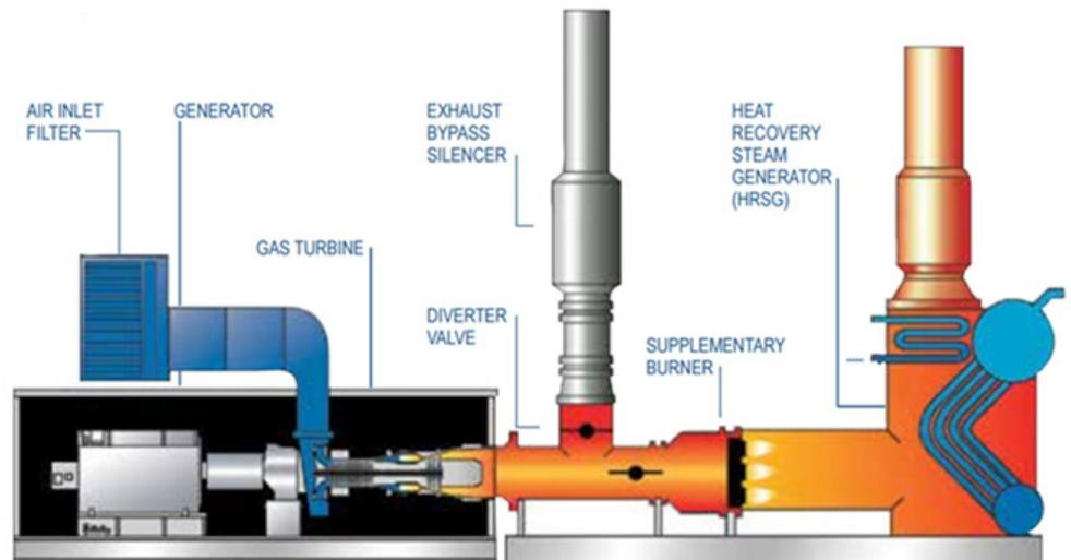
Figure 1. Gas turbine configuration with heat recovery.
