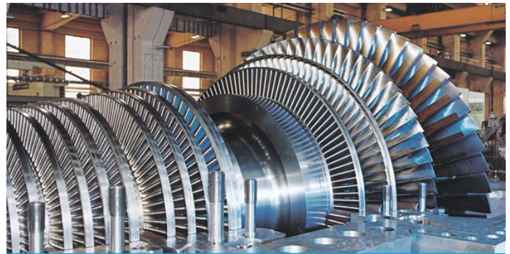
Interior view of steam turbine blades. Photo courtesy of Siemens
